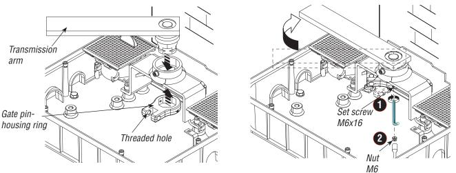
Note: for the right side gearmotor, assemble the gate pin with the pin-housing ring so that is symmetrical to the left side one, see illustration.
